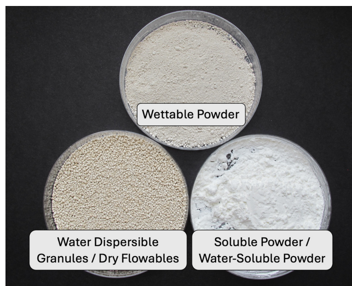
Figure 2. Wettable powders, water dispersible granules, and soluble powders are examples of concentrated dry formulations which are mixed with water and applied as a spray.
