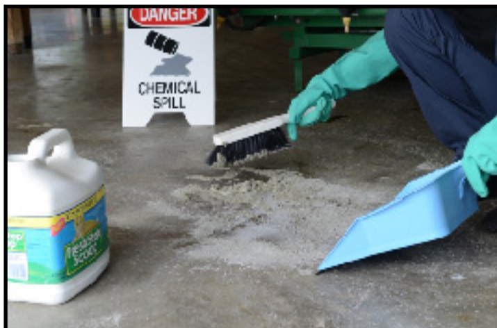
Figure 1. An example of spill clean up. Pet litter has been spread over a liquid spill and is being swept up for disposal.
