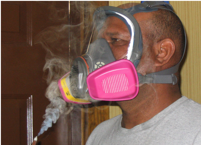
Figure 1. Qualitative respirator fit test using irritant smoke.
