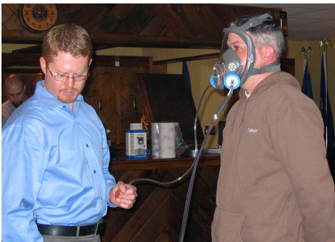
Figure 2. Quantitative respirator fit test.
