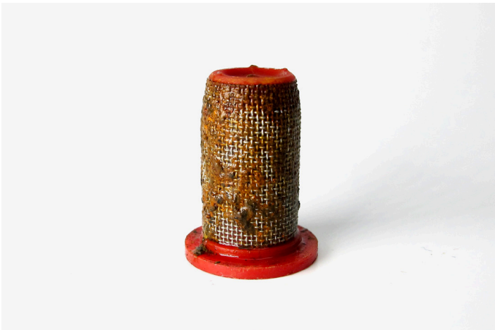
Figure 3. A nozzle strainer that has been damaged over time from constant contact with water.
