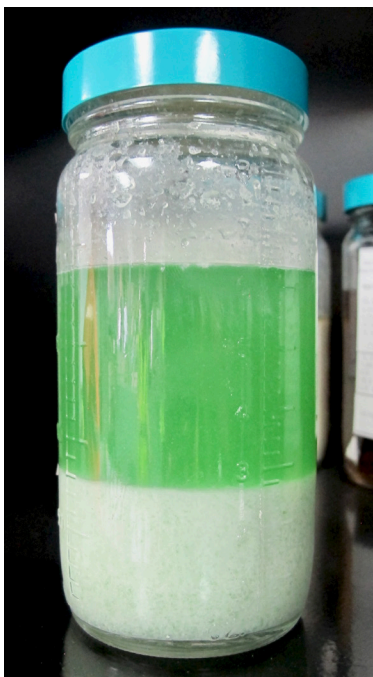
Figure 1. This jar test shows an example of product incompatibility — the mixture has separated. After adding a compatibility agent, repeat the jar test to see if the products are now compatible.
