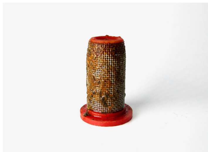
Figure 2. A nozzle strainer that has been damaged over time from constant contact with water.
