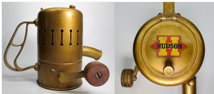
Figure 4. Side view (left) and top view (right) of Hudson Rotary Duster, circa late 1950s to early 1960s.
