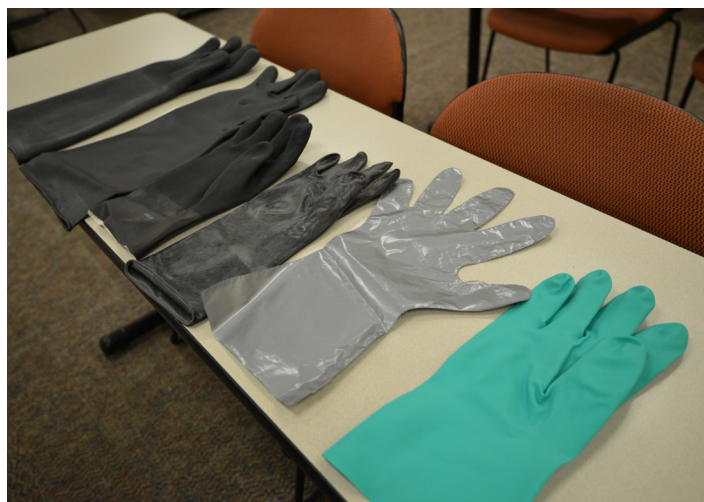
Figure 3. Types of chemical-resistant gloves. Displayed from left to right are natural rubber, neoprene, fabric-lined (not safe for pesticide use), butyl, barrier laminate, and nitrile.
